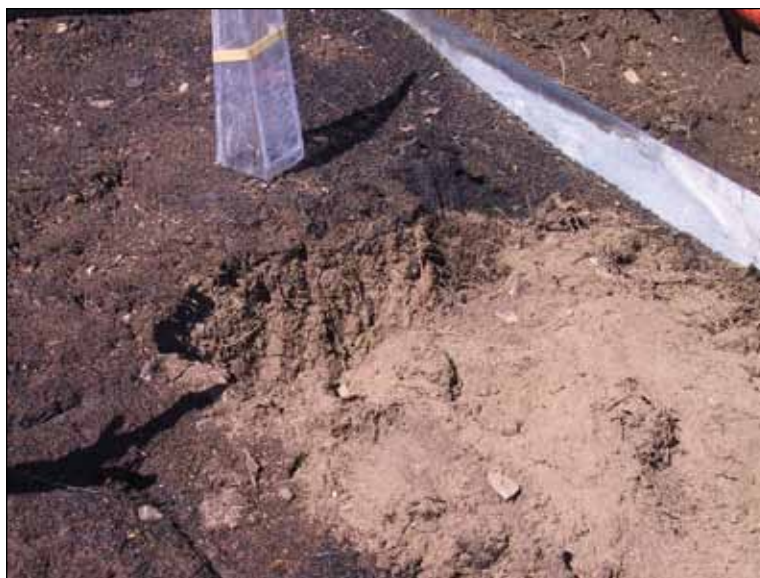
Figure 19 —Dry soil underneath a 2- to 3-cm thick layer of water repellent soil observed immediately after application of 85 mm of rainfall (see Pierson et al. 2008b) over a 1-h period following the Breaks Prescribed Fire, Reynolds Creek Experimental Watershed, Idaho. Soils were strongly water repellent at the mineral soil surface and to a depth of 2 to 3 cm immediately before and after the prescribed fire (photo: USDA Agricultural Research Service, Northwest Watershed Research Center).
